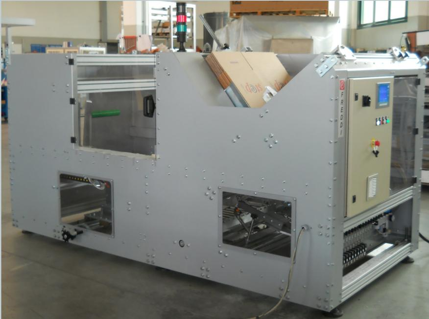
**FC/12 CASE ERECTOR IS DESIGNED TO ERECT CFC CORRUGATE AMERICAN CARTON WITH DIFFERENT SIZES, MAIN FEATURES OF THE MACHINES ARE USER FRIENDLY CONCEPT, RELIABILITY AND RAPID CHANGE SIZE FROM SMALL TO BIG CARTONS.**
