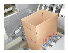
FC/12 case erector has a modular concept, this guarantee great flexibility; in fact same machine could be equipped as a single case erector having both tape or hot glue closure, in alternative same machine could be equipped with product layer preparation and picking head becoming a case packer mono
