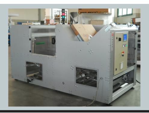
FC/12 CASE ERECTOR IS DESIGNED TO ERECT CFC CORRUSATE AMERICAN CARTON WITH DIFFERENT SIZES, MAIN FEATURES OF THE MACHINES ARE USER FRIENDLY CONCEPT, RELIABILITY AND RAPID CHANGE SIZE FROM SMALL TO BIG CARTONS.
