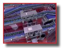
The machine is normally fixed on specific bottling lines with metallic crown cap or twist-top for bottles lockup. This process has as aim the elimination of any glass shreds and any lying bottles on the conveyor.
