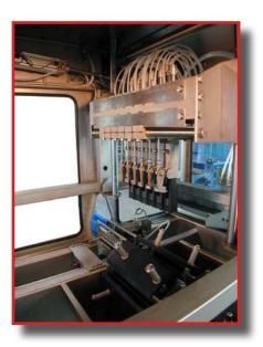
The machine is dedicated to the bottling industry, on the line for the evacuation and recovery of products. The discarded product is sent to the machine which takes off the lids and empties the glass bottles (closed with a crowned metal cap) or to cut and empty tins.
